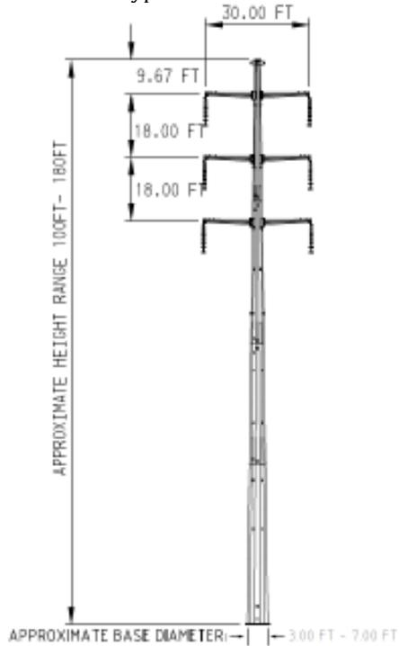
Typical 220-kV Double Circuit LST
