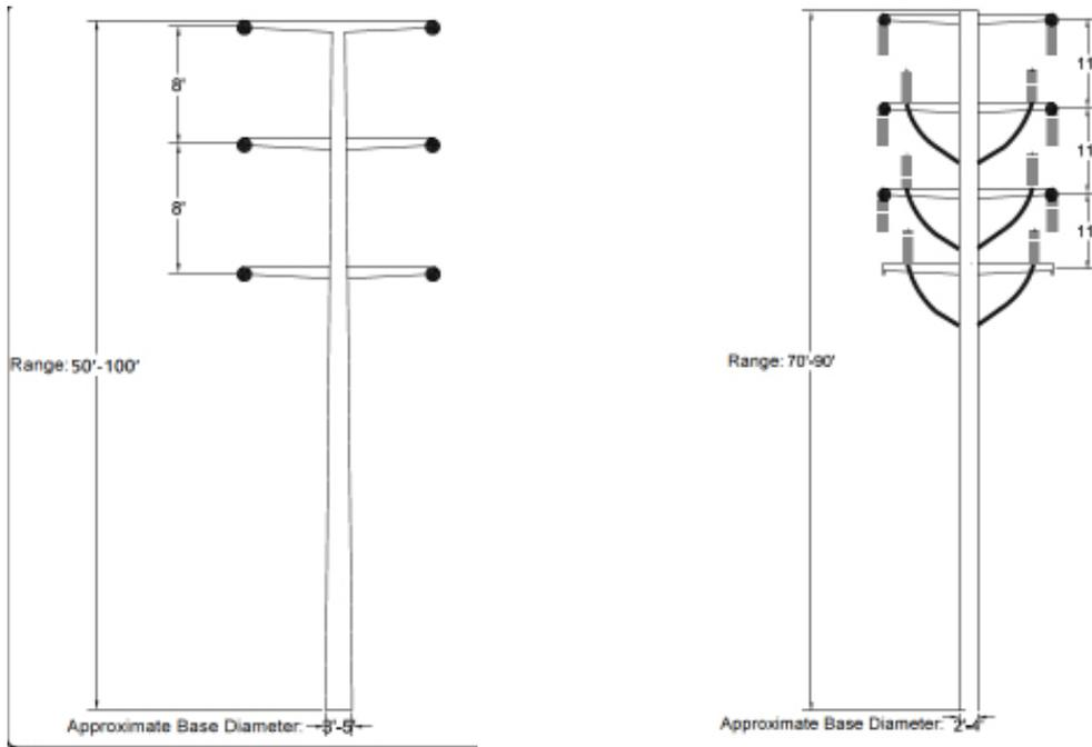
Typical 66-kV Double Circuit TSP (no underbuild)
