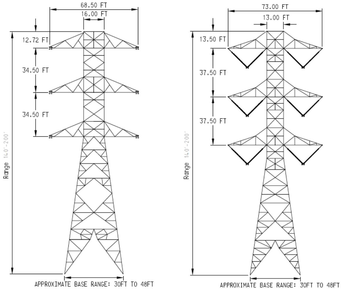
Typical 500-kV Double Circuit LST
